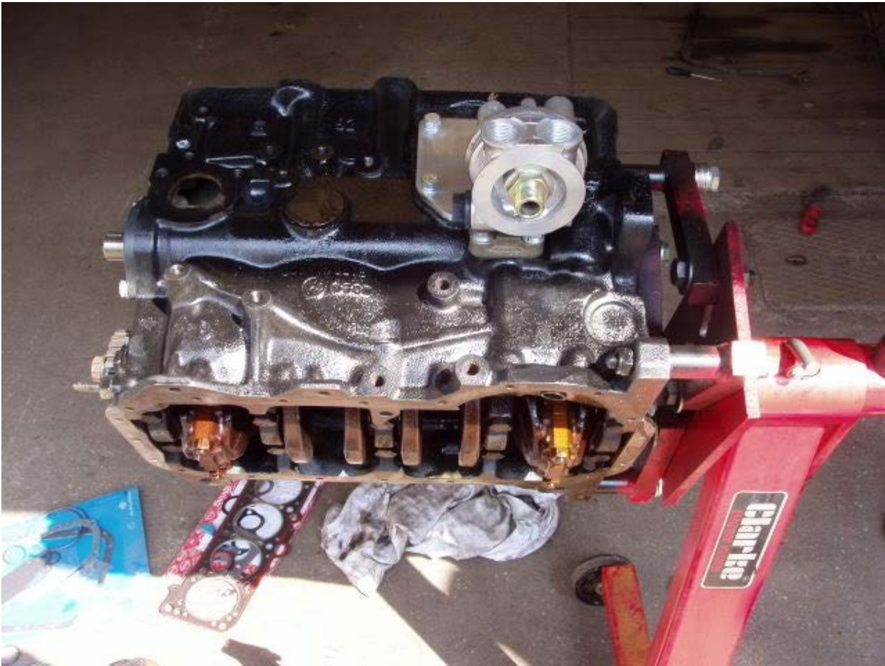
2e block with oil cooler adaptor and blanking plate attached
