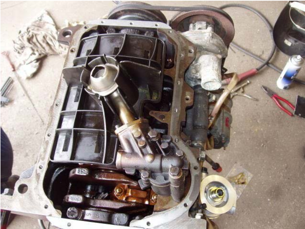
oil pump with a mk3 gti baffles attached
