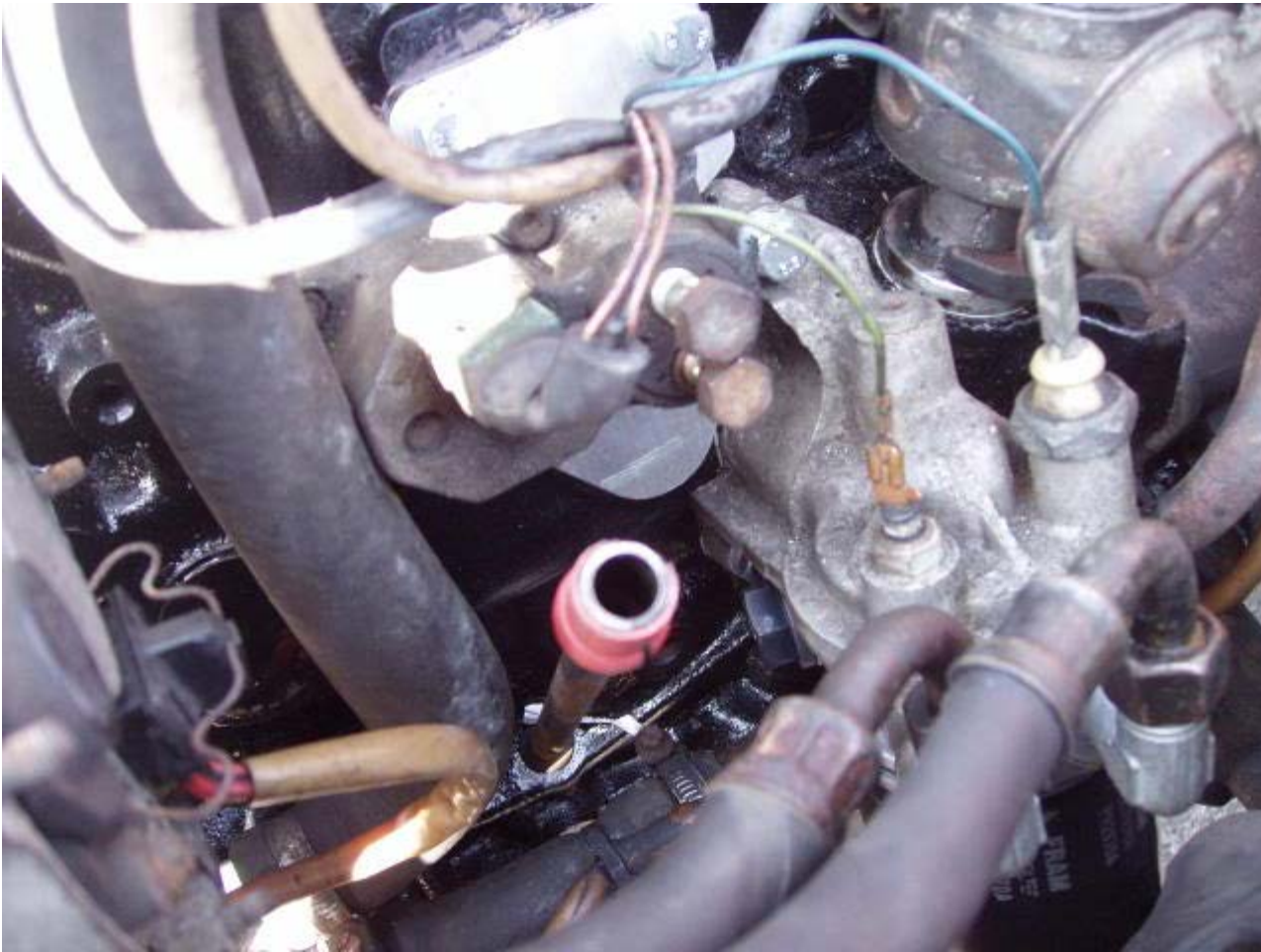
WUR mounted on blanking plate
